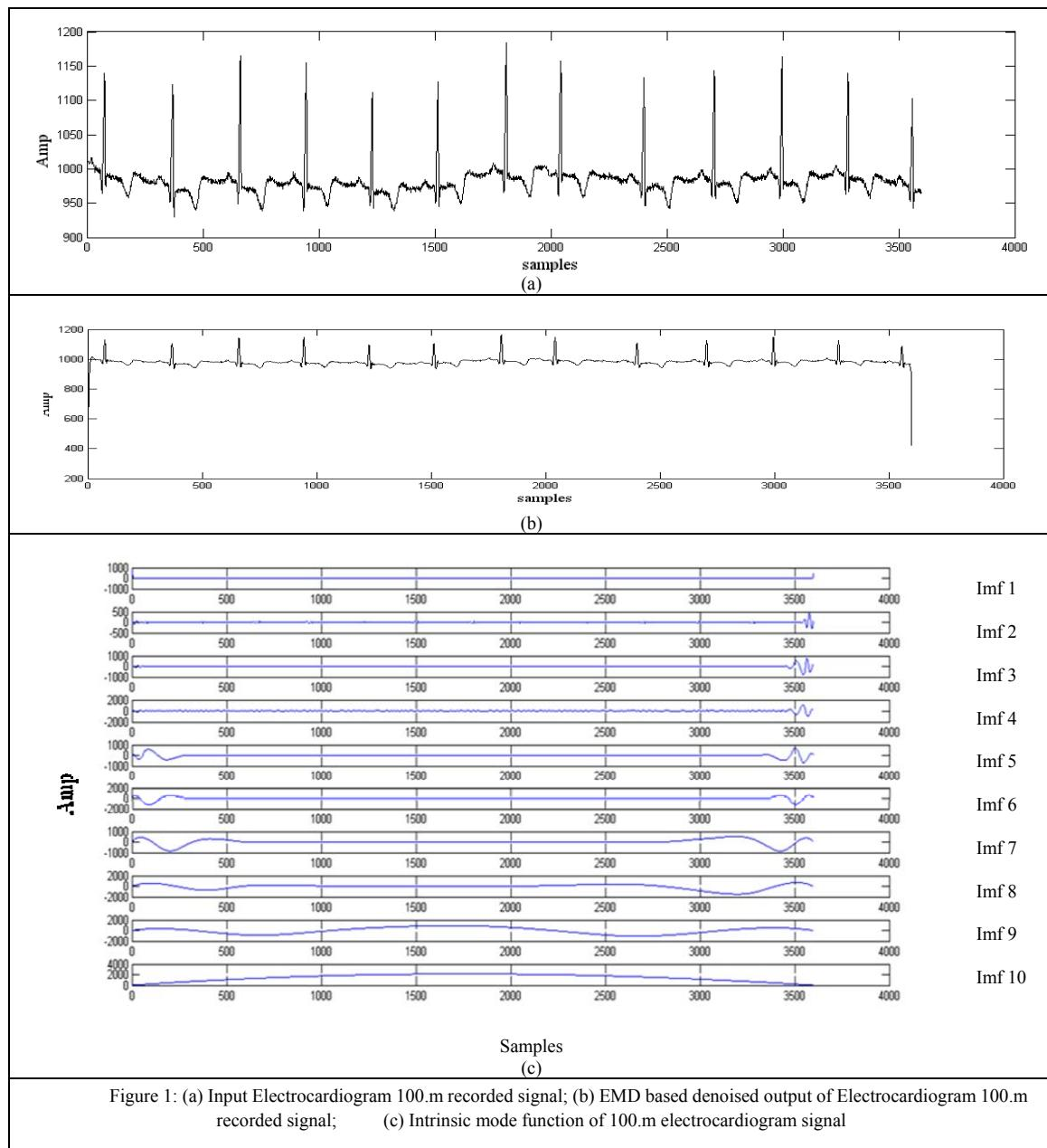
Figure 1: (a) Input ECG signal; (b) EMD based denoised output; (c) 10 IMFs of the ECG signal
